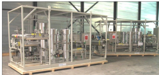
Above three extended gas skids with KO-vessel, 2x 100% particle and 2x 100% coalescing filter, electric heater (with thyristor control panel), stainless steel piping & vessels and a flow meter
