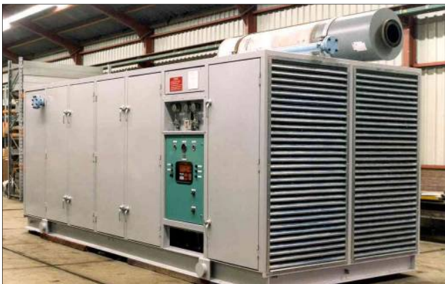
Typical tailor-made diesel engine driven (back-up) compressor package including an oil-flooded screw.
