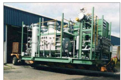
Eltacon off-gas compressor package. Year of construction 1995
