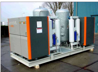
Instrument air system including vane-type compressors
