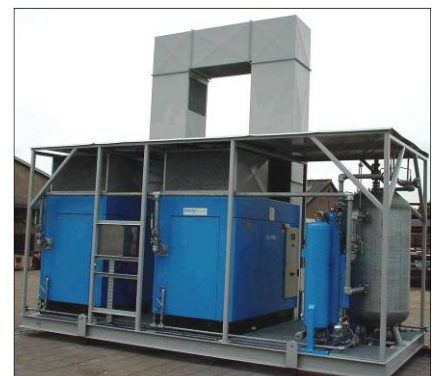
Instrument air system including oil-free screw compressors.
