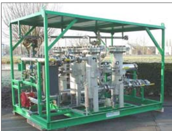
Above three extended gas skids with KO-vessel, 2x 100% particle and 2x 100% coalescing filter, electric heater (with thyristor control panel), stainless steel piping & vessels and a flow meter
