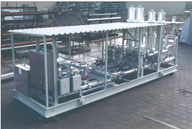
Above at the left gas pressure reduction station with 2x 100% streams for gas turbine and auxiliary boilers. Gas flow 50.000 nm 3 /h, footprint 8,5 x 2,5 meters.
