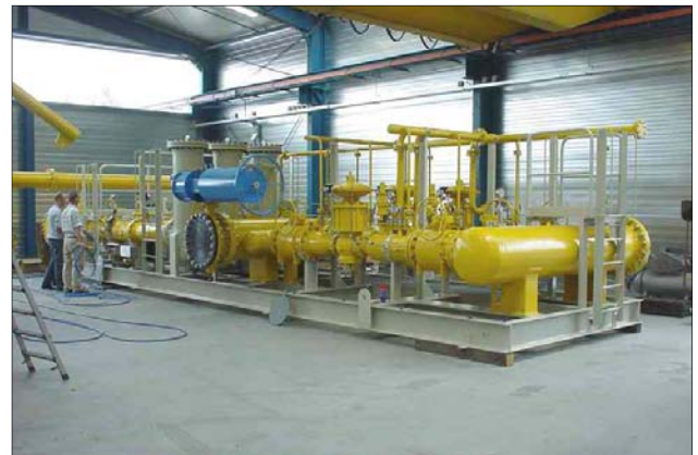
Above three extended gas skids with KO-vessel, 2x 100% particle and 2x 100% coalescing filter, electric heater (with thyristor control panel), stainless steel piping & vessels and a flow meter
