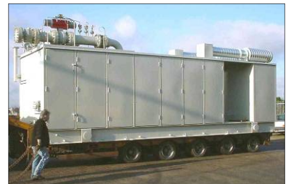
Package with 1130 kW E-motor. 20.000 nm 3 /h from 4 to 26 barg.
