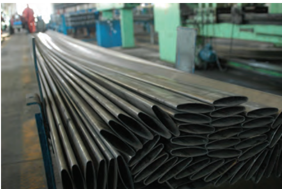
Carbon steel bare tubes waiting to be finned
