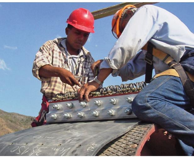
Splicing of steel-reinforced belt
