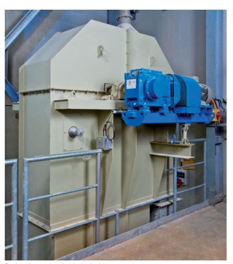
Bucket elevator head with single drive
