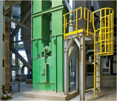
Elevator boot with parallel tensioning device
