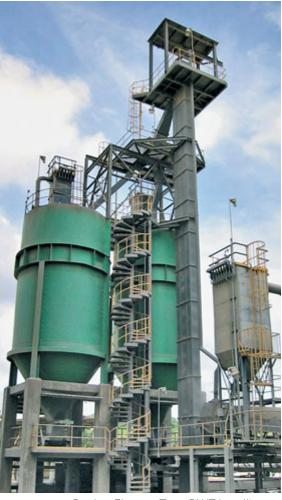
Bucket Elevator Type BWZ handling pozzolana and limestone
